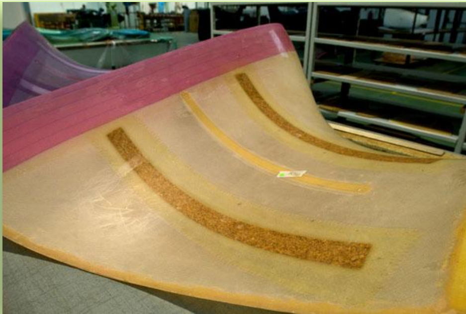
Fabric strips replaced in winglets by CORECORK NL10
